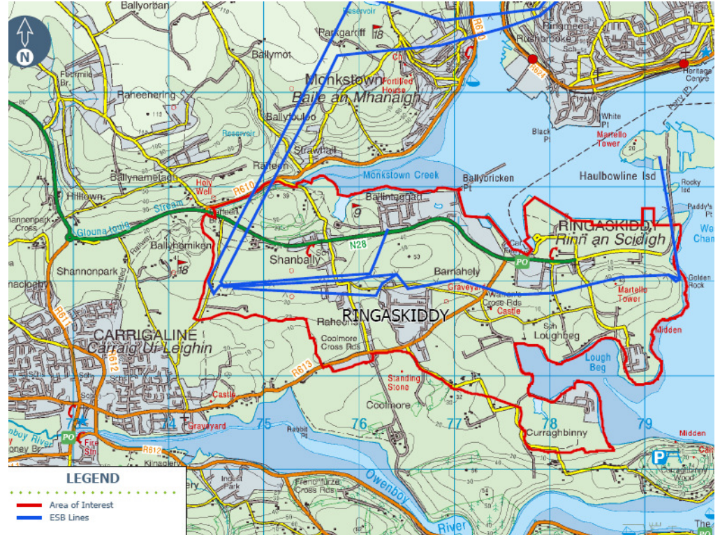
Figure 6.3: Overhead power cables in the Ringaskiddy area
