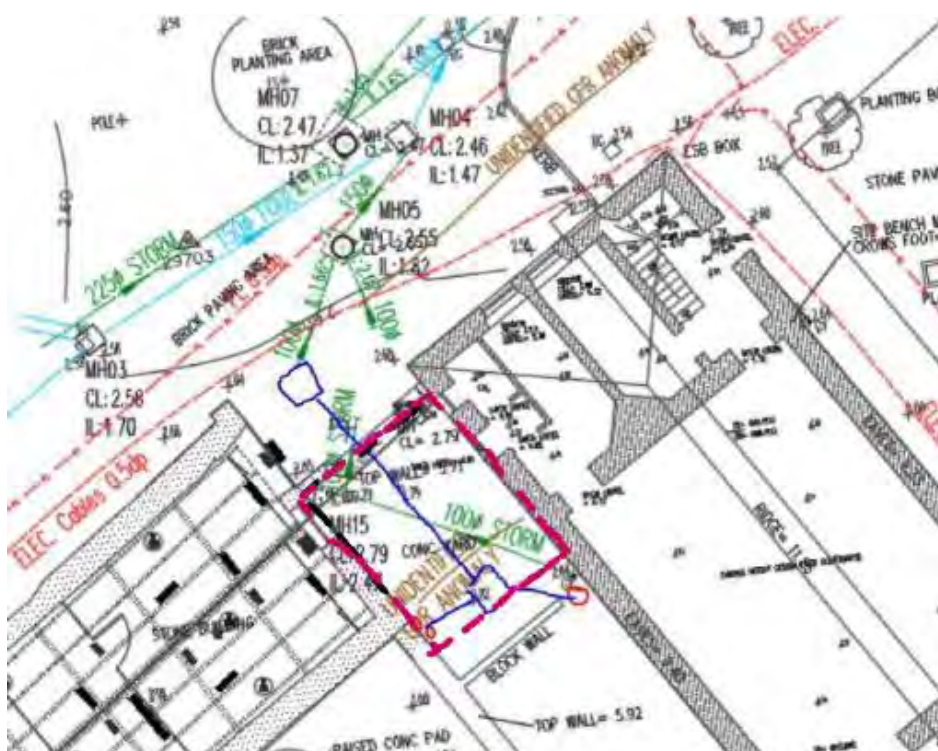
Figure 4-3 Proposed drainage works at extension
