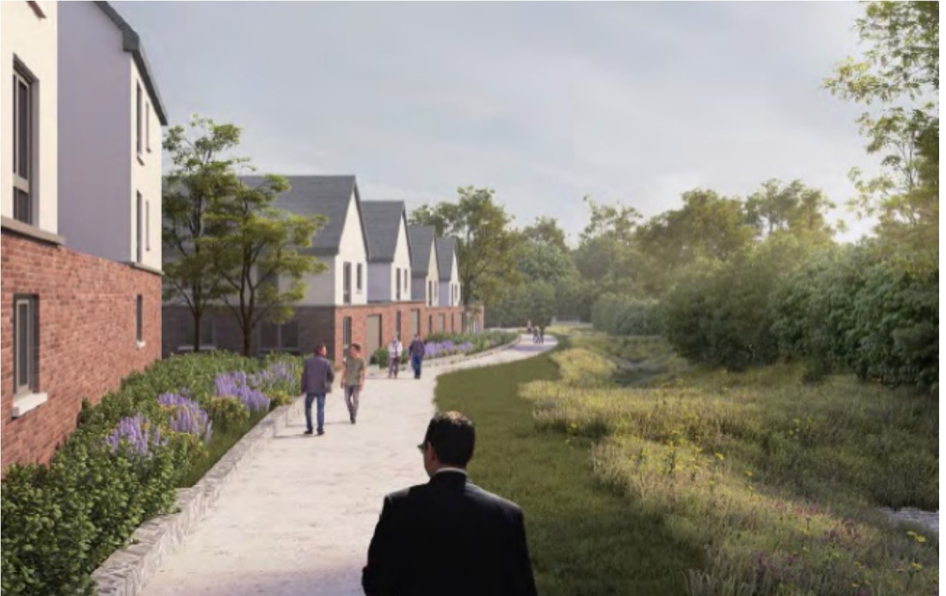
Fig 3.11 Visualisation illustrating how hedgerow can be incorporated into the SuDS drainage design augmenting a riparian corridor Source: Landscaping and Biodiversity Guide for New Developments (Cluid Housing)
