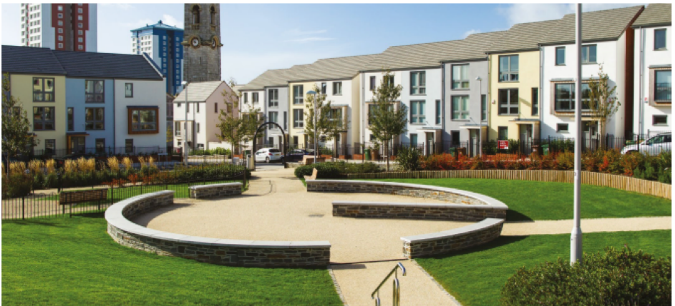
Fig 6.18 Natural surveillance of public open space – Source: Secure by Design Guide (2023 – UK)
