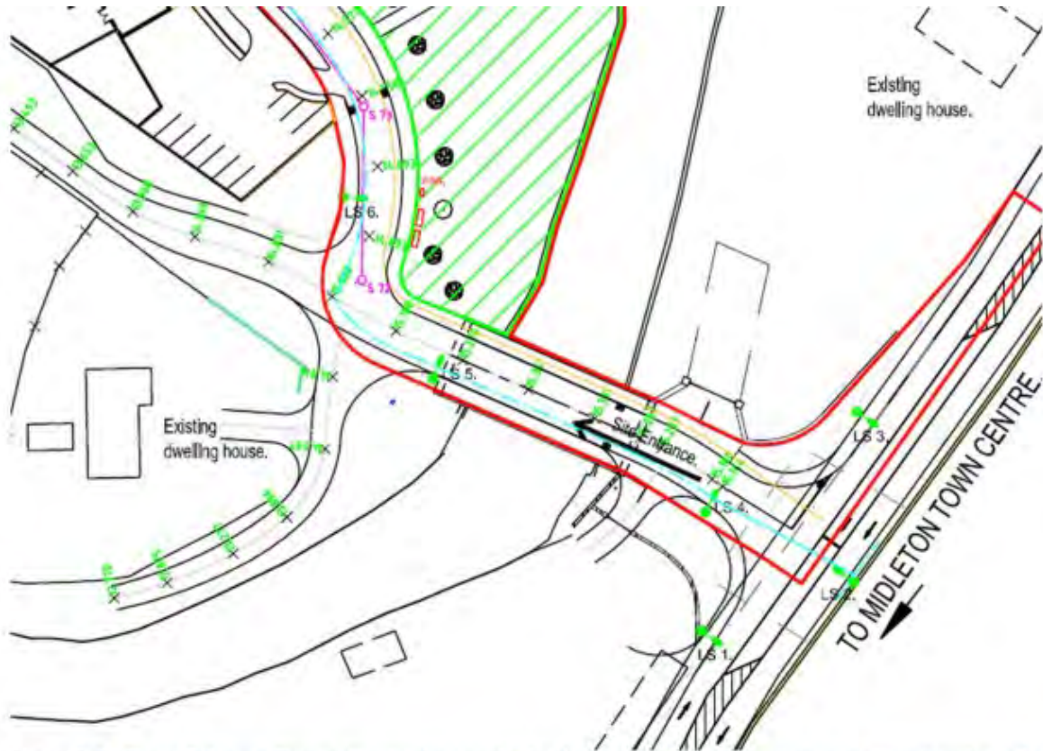
Figure 2: Tir Cluain Taking in Charge drawing (zoomed in to show revised access/egress arrangement and private bridge removed)
