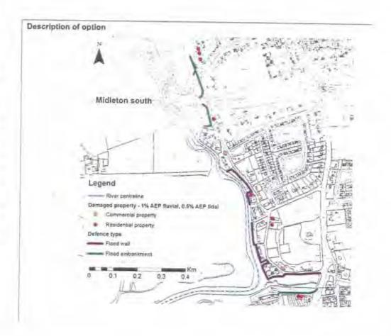
Figure 6.8 Draft Lee CFrams Study Option for Flood Protection at Bailick/Ballinacurra, February 2010, Appendix E
