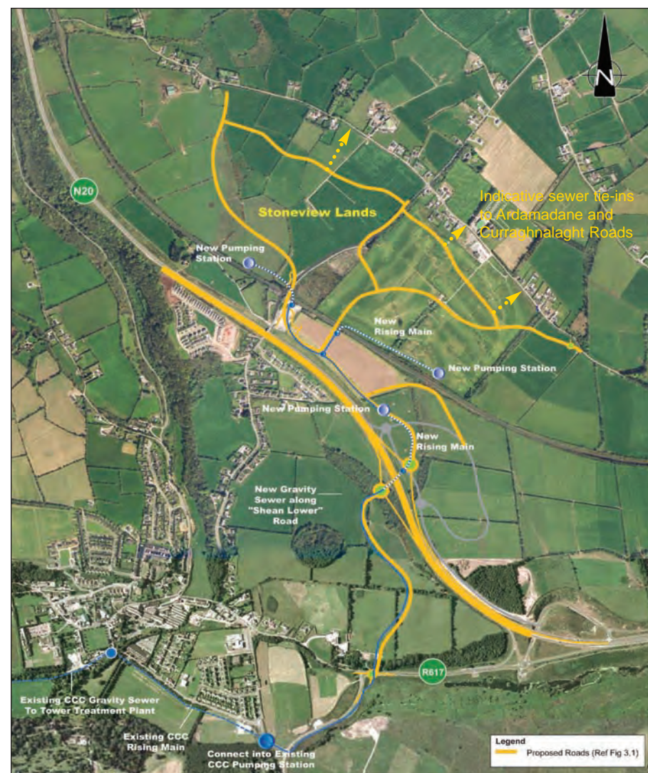
Figure 23: Proposed Foul Drainage Layout
