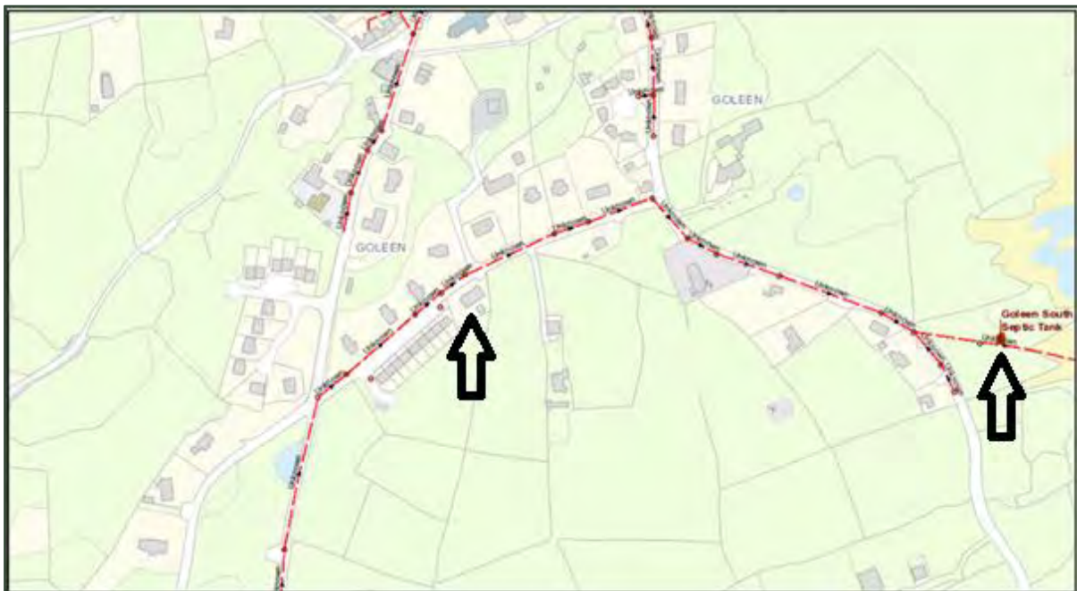
Figure 3.2 – Existing foul water networks servicing the proposed site. Following on-site pre-treatment, foul water will flow eastward to ‘Goleen South Septic Tank’.
