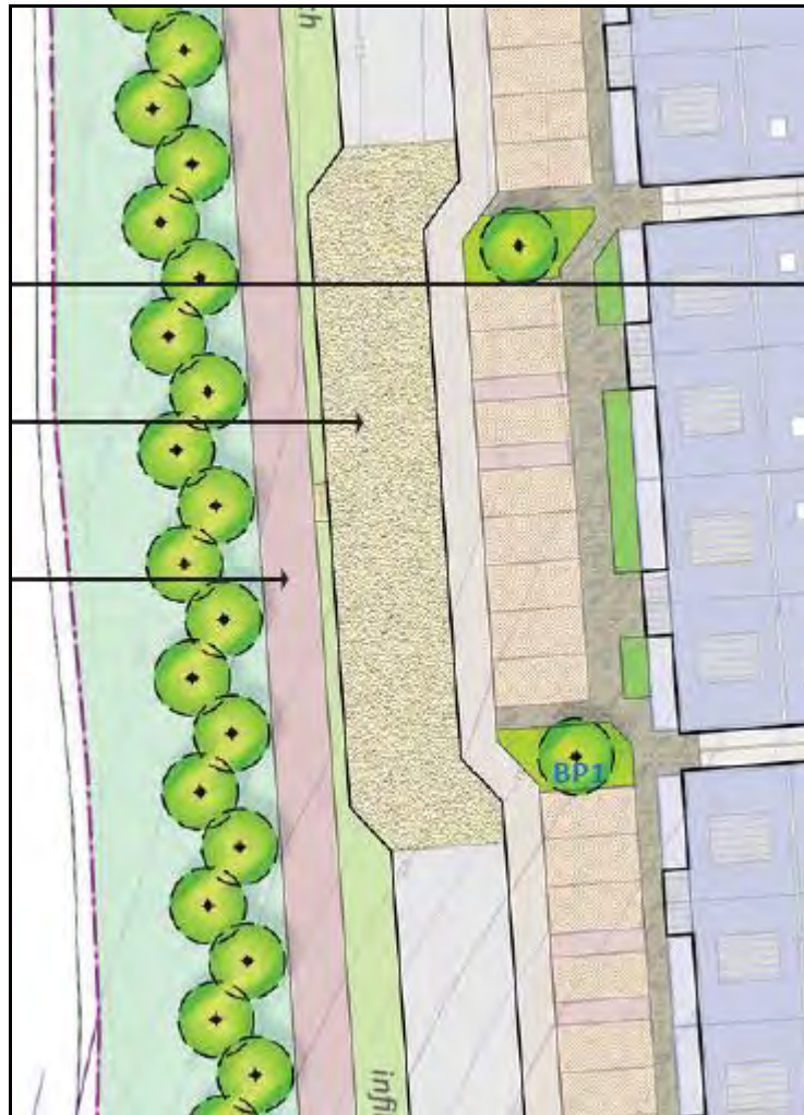
Figure 23: Sharp kerb edges at chicane arrangement
