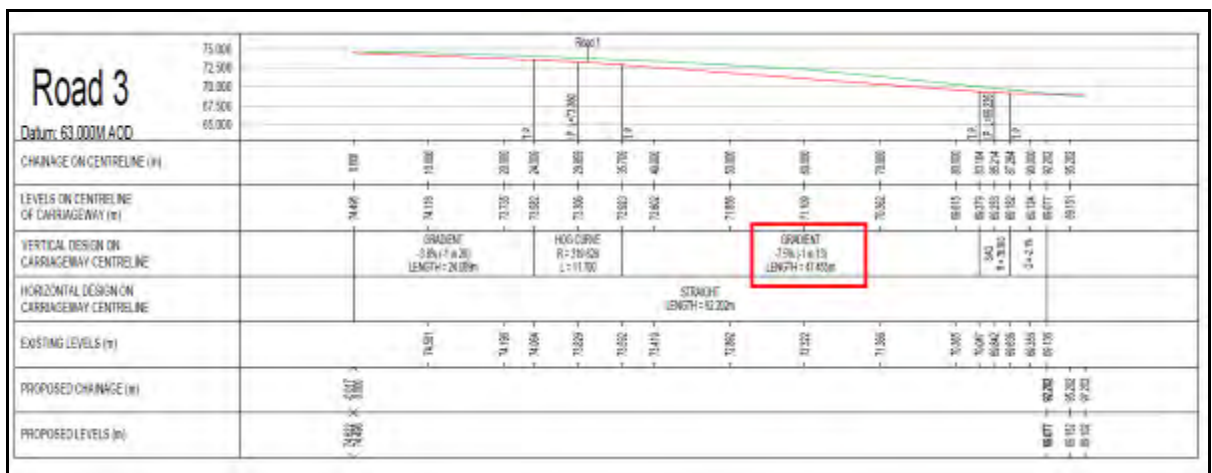
Figure 27: Step gradient on Road 3
