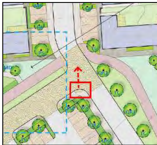
Figure 35: Poorly Orientated Tactile Paving Warning surfaces absent at intersections of footways/shared surfaces
