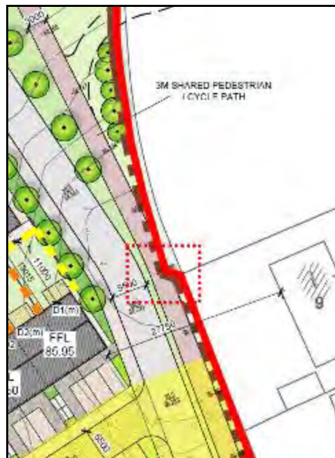
Figure 42: Boundary (2m high mesh fencing & vegetation) encroaching into narrow shared surface
