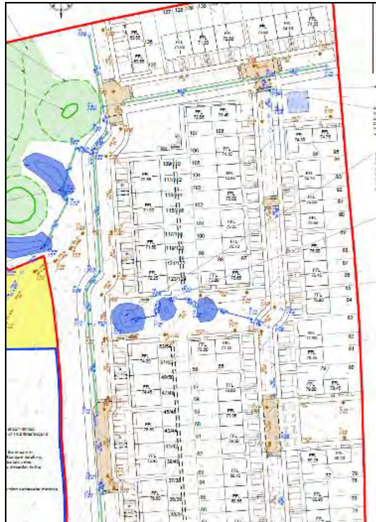
Figure 22: Extract from plan showing different surface types at junctions & ramps And the location of water hazards
