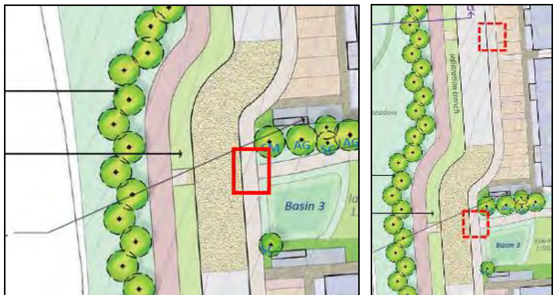
Figures 33 & 34: Incomplete Tactile Paving Detail at informal crossing point
