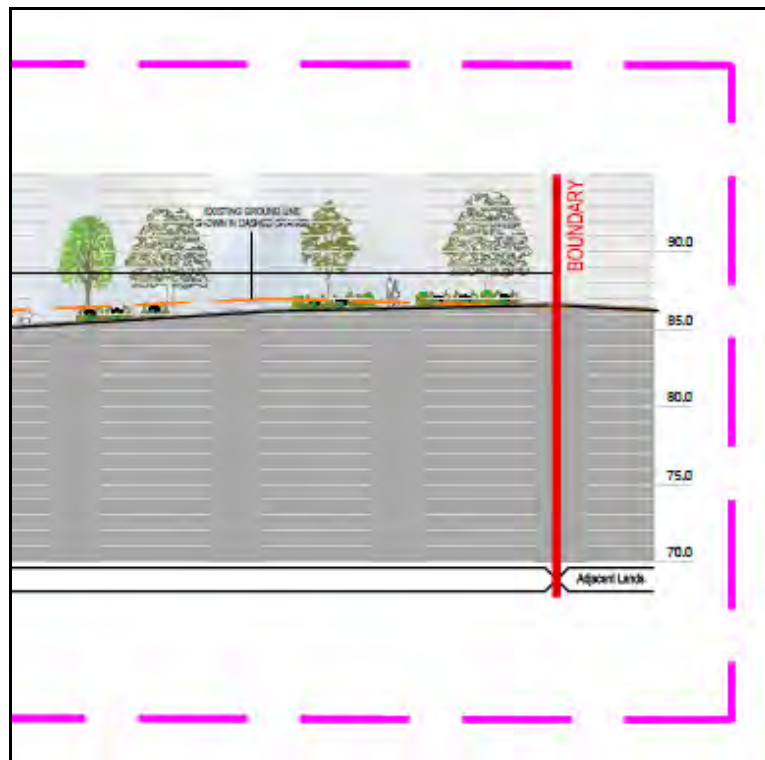
Figure 17: Extract from section E-E showing crest curve at southern Tie-in on Road 1
