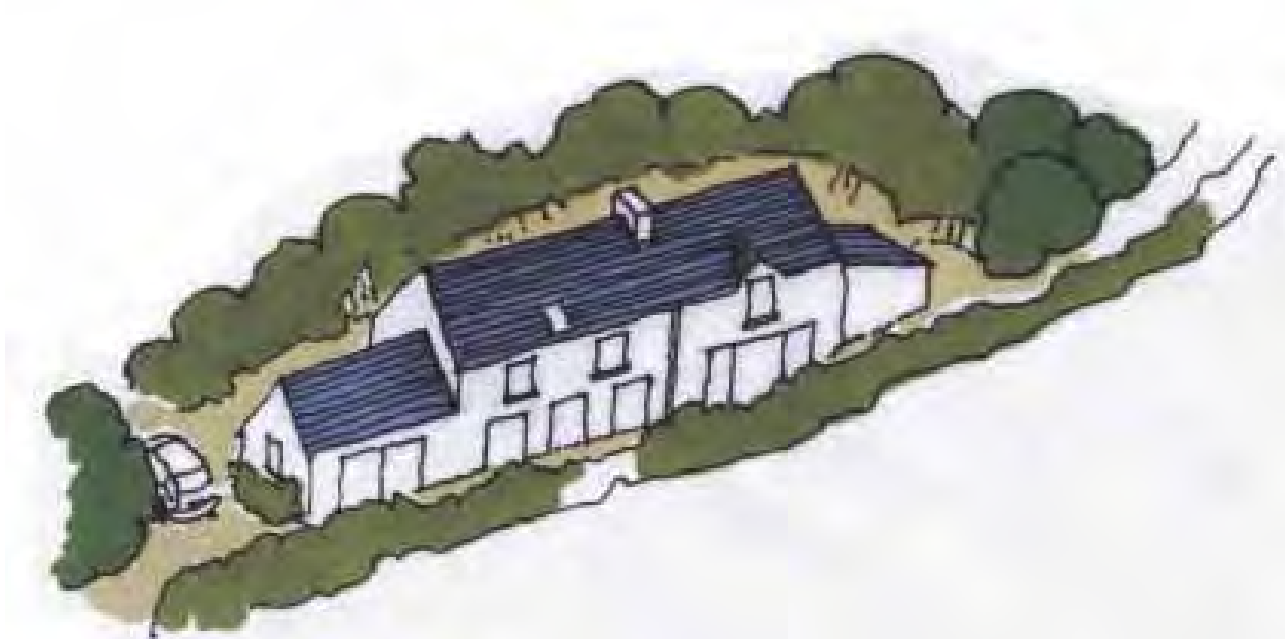
Extensions and additions should be directed to the gable end or rear elevation
