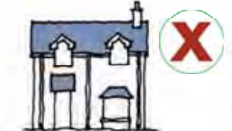
House too small for so many RWP's
