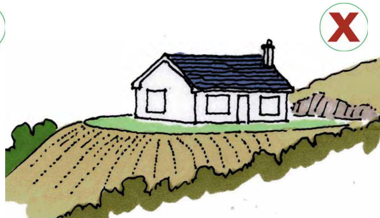
Avoid mounding up to form a flat site. This makes the house more conspicuous in the landscape, reduces its ability to retain heat/energy and exposes the exterior to the worst effects of weathering
