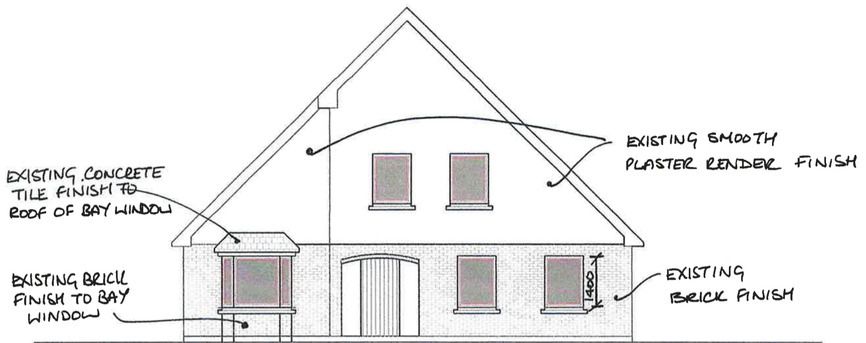
Existing Front Elevation
