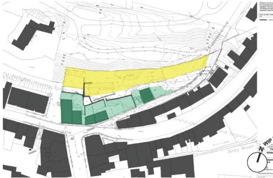
01. Diagram highlighting existing site levels highlighting 2 tiers with approx 4-5m change in level. Note upper yellow section is gently sloping as it formed part of the old railway platform.
