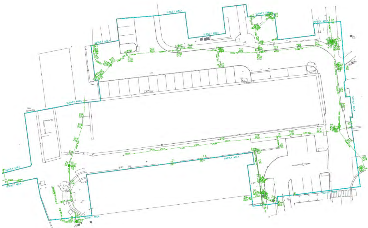
Figure 1.2: Below ground utility survey drawing - Existing storm sewer (marked in green colour)
