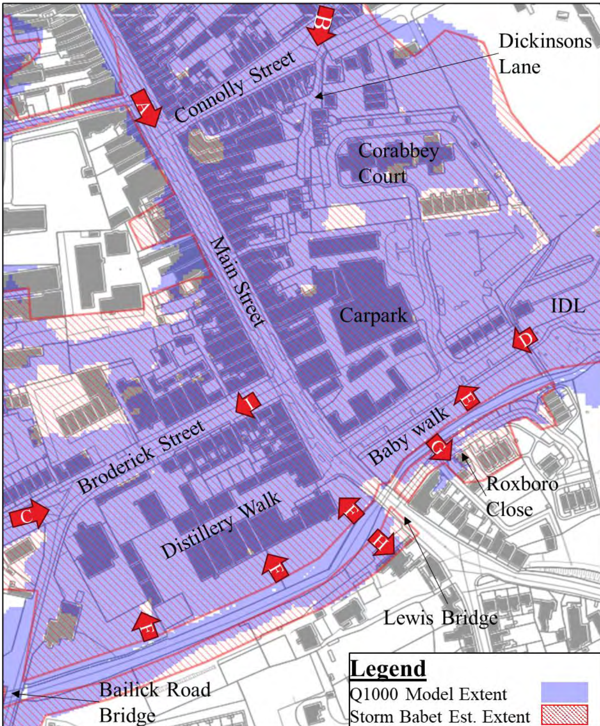
Figure 71: Lower Main Street/ The Babys Walk: Existing Flood Mechanisms
