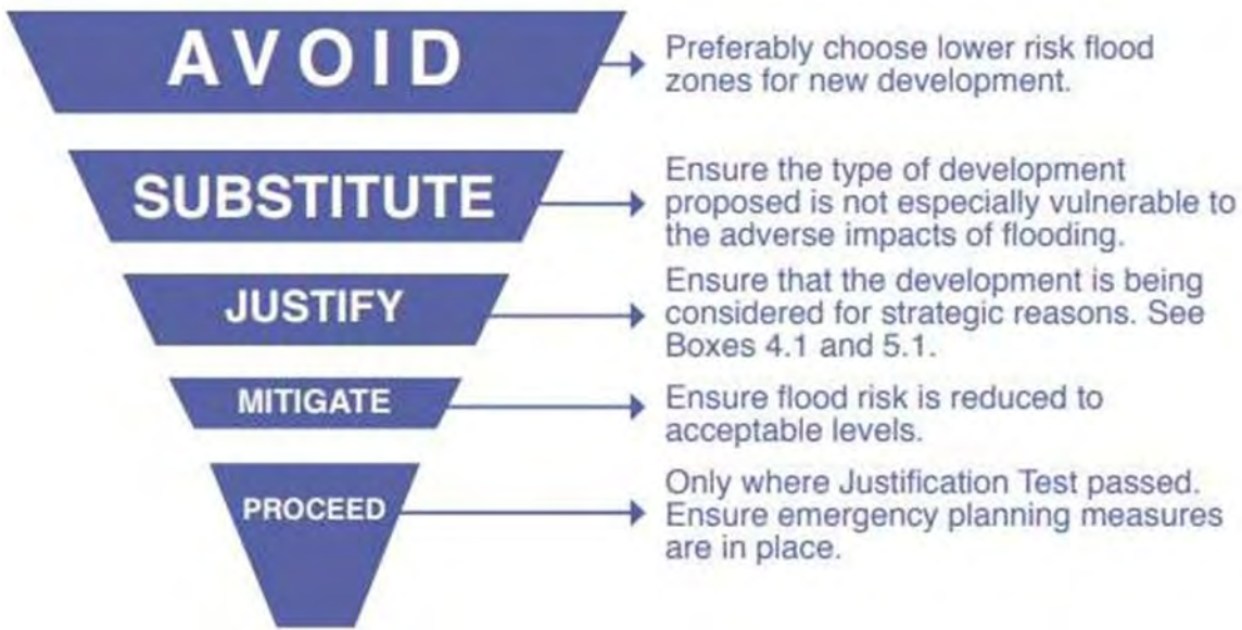
Figure 1.5: Sequential approach principles in flood risk management
