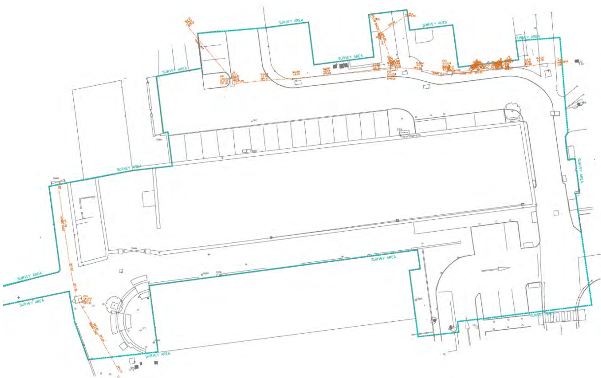
Figure 2.1: Below ground utility survey drawing - Existing foul sewer (marked in brown colour)
