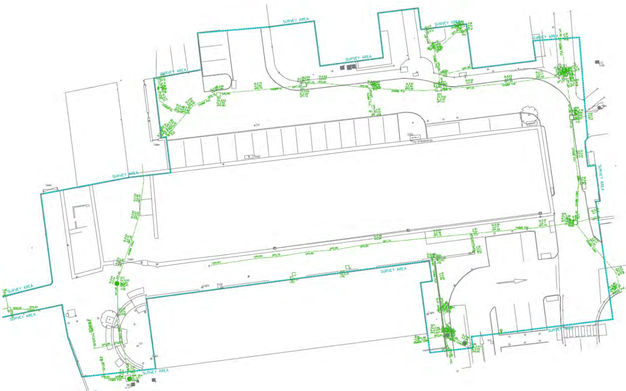
Figure 3.1: Below ground utility survey drawing - Existing storm sewer (marked in green colour)
