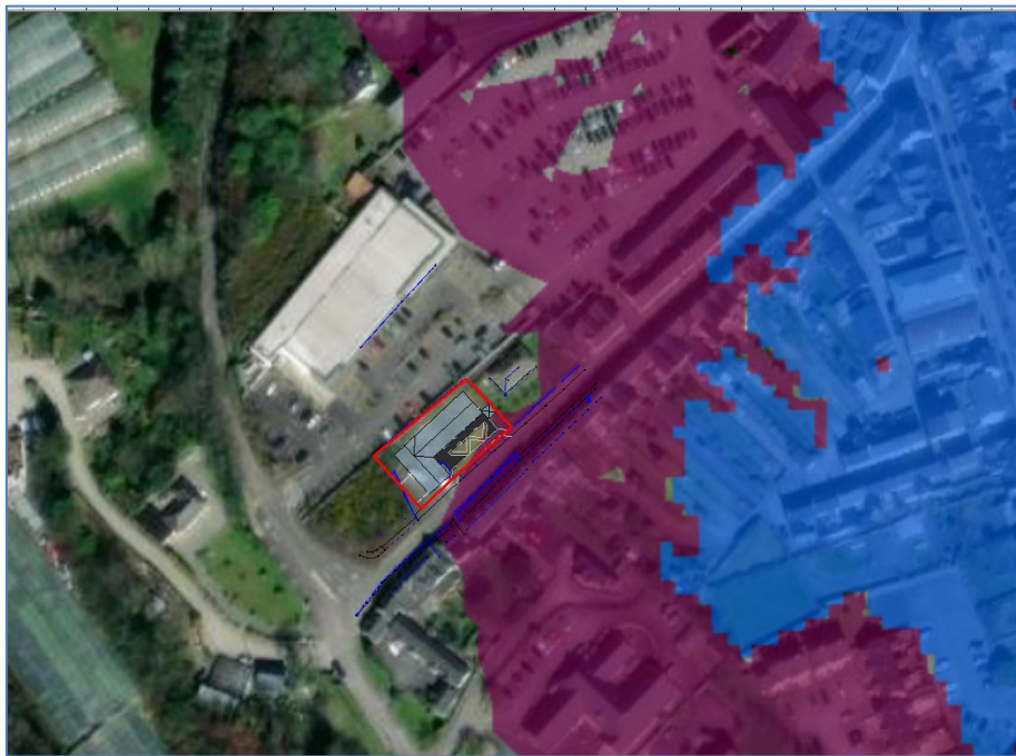
Figure 1.5 - Site overlay on CDP 2022 map (Zone A light blue, Zone B magenta)
