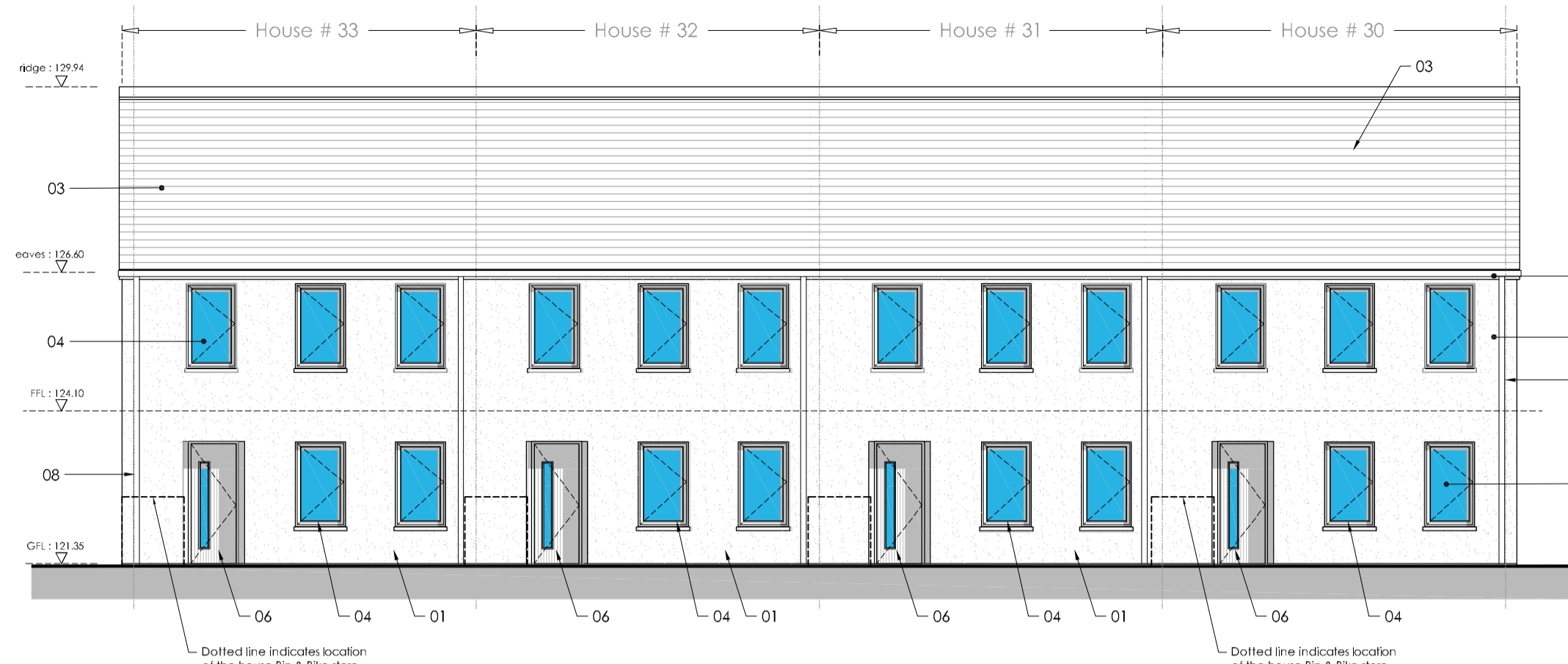
2-Bed Houses - Front Elevation (Southeast) Scale 1:100 @A1
