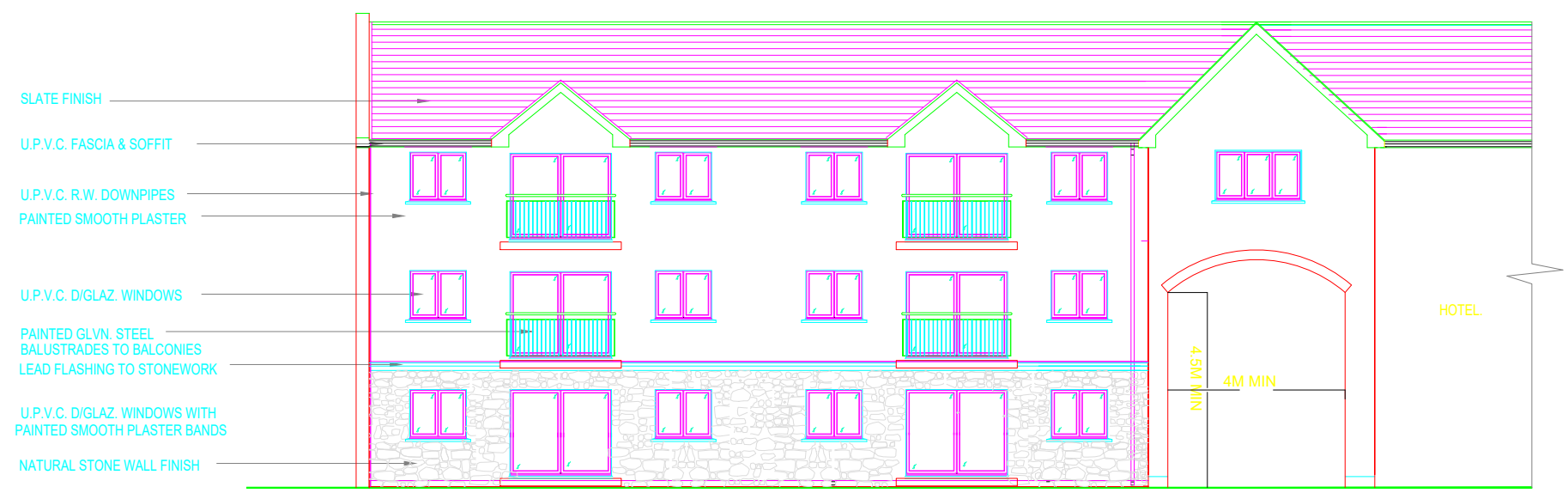
APARTMENT BLOCK 1 - FRONT ELEVATION.
