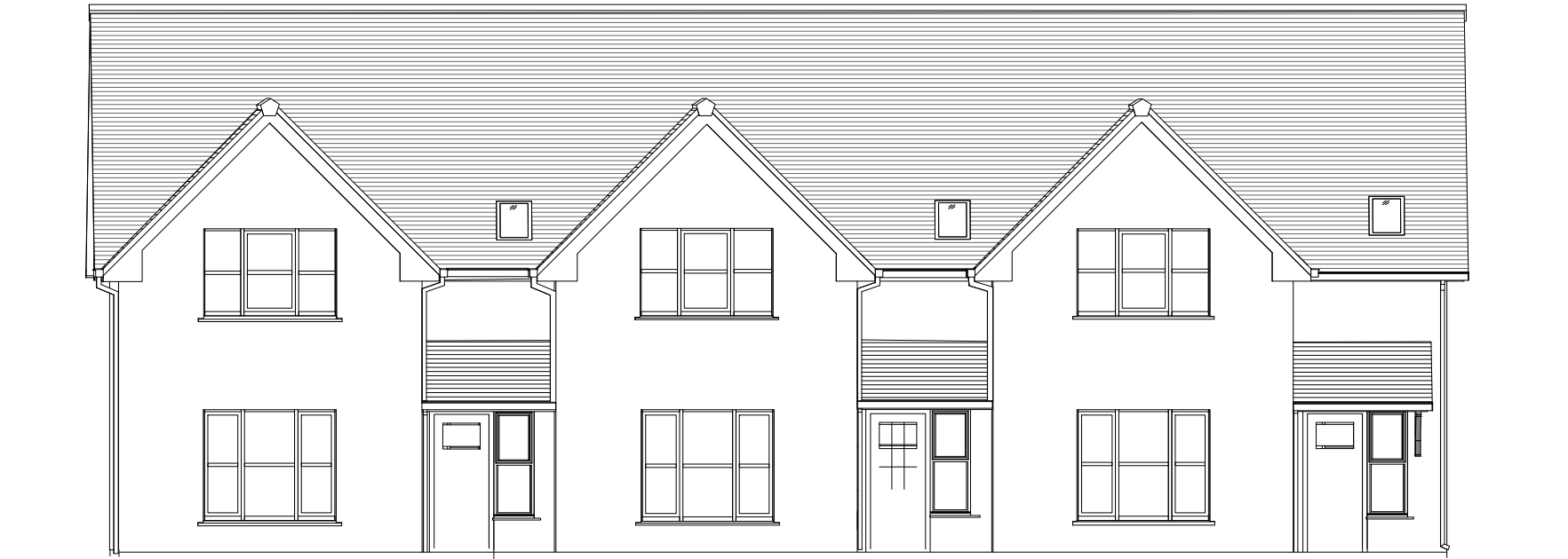
Front Elevation - Typical End of Terrace
