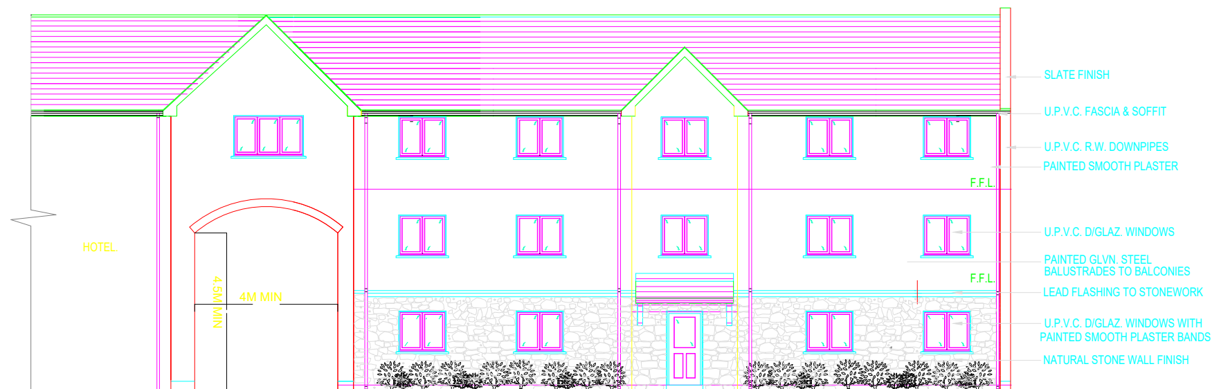
APARTMENT BLOCK 1 - REAR ELEVATION.
